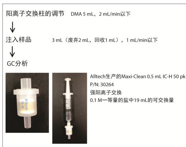
图 2 用阳离子交换柱进行预处理的步骤 Procedure for Pretreatment Using Cation-Exchange Cartridge
